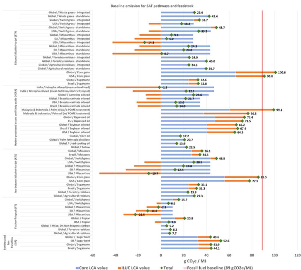
Figure 18: LCA emissions for CORSIA SAF pathways and feedstock compared to CORSIA fossil fuel reference value (89 g CO 2 e/MJ)
