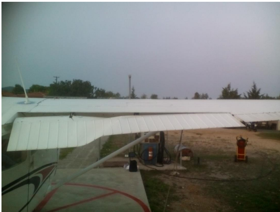
Figure 10 Flap deformation following asymmetric flap retraction
