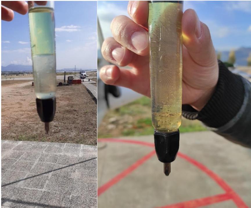
Figure 7 Different types of fuel contamination
