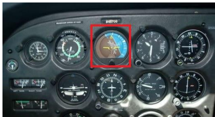
Figure 8 Artificial Horizon failure
